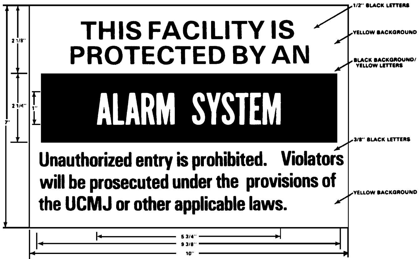
Figure F-1. Sample Intrusion Detection System sign
