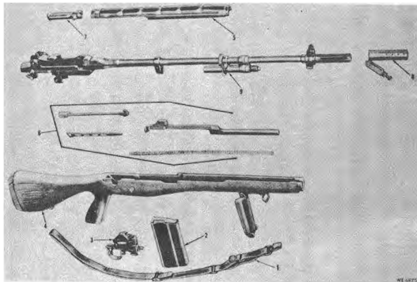
Figure 3-2. Weapon field stripped (M14A1).
