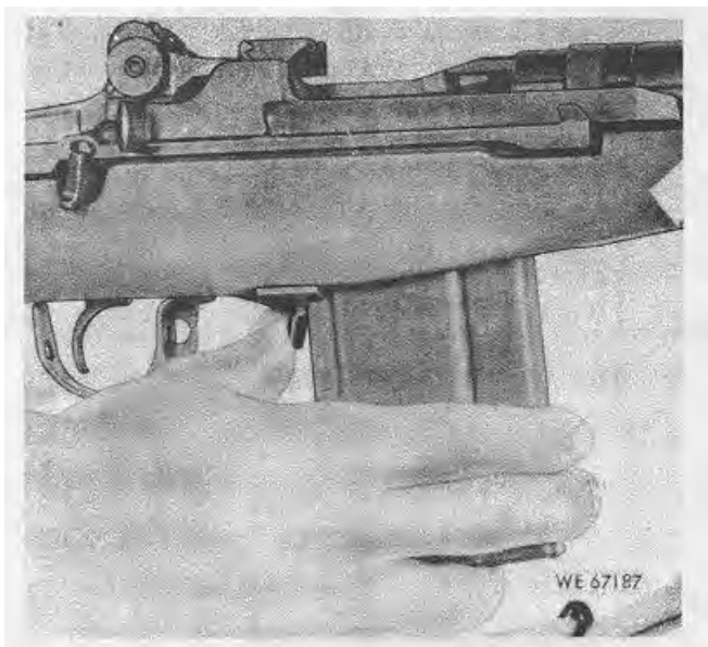
Figure 2-12. Removing magazine from rifle.
