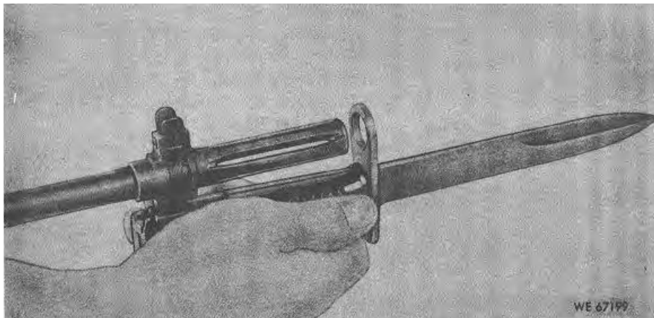
Figure 2-17. Installation/removal of bayonet-knife.
