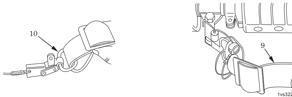
Figure 11. Securing Swivel and Lanyard.
