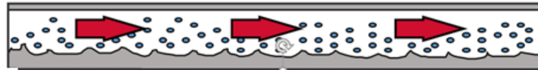
ANNULAR FLOW (HIGH GAS VELOCITY)
